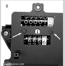
Line up the small gear you just removed and reinsert into position. You may wish to move the reset shaft back and forth slowly to ensure smooth operation, but no lubrication is necessary or recommended. Next, reinstall the trip reset shaft assembly (with the new shaft in position) and replace the two 3/16" screws to hold it in place.
